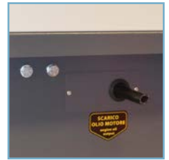
External oil drain point allow to change oil easily
