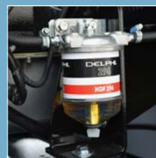
Fuel/Water Separator Filter removable for places where space is limited
